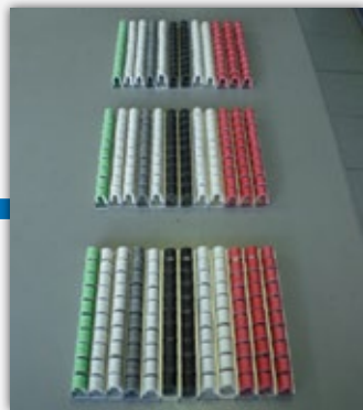
Samples prepared for ageing in oven at different temperature.
